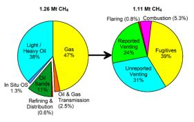
Figure 3 - 2014 Methane emissions from the oil and gas sector in Alberta (ECCC's National Inventory Report). The left pie chart = contributions from different upstream production types; the right pie chart illustrates the emission types from natural gas and conventional oil production (excluding mined oil sands).
