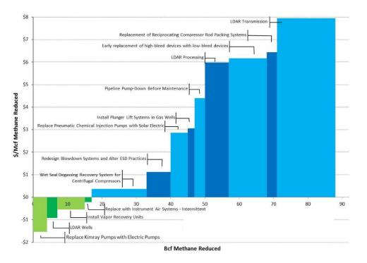
Figure 7 - Marginal Abatement Cost Curve for Methane Reduction
