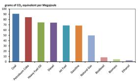
Figure 10 - Carbon Intensity Comparison of Various Fuel Types ("Canada's Energy Future" NEB 2016)
